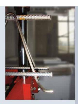
Hydraulically actuated girder shears for burr-free cutting in the upper or lower weld joint. The girder shears are positioned by means of a motor-driven system.
